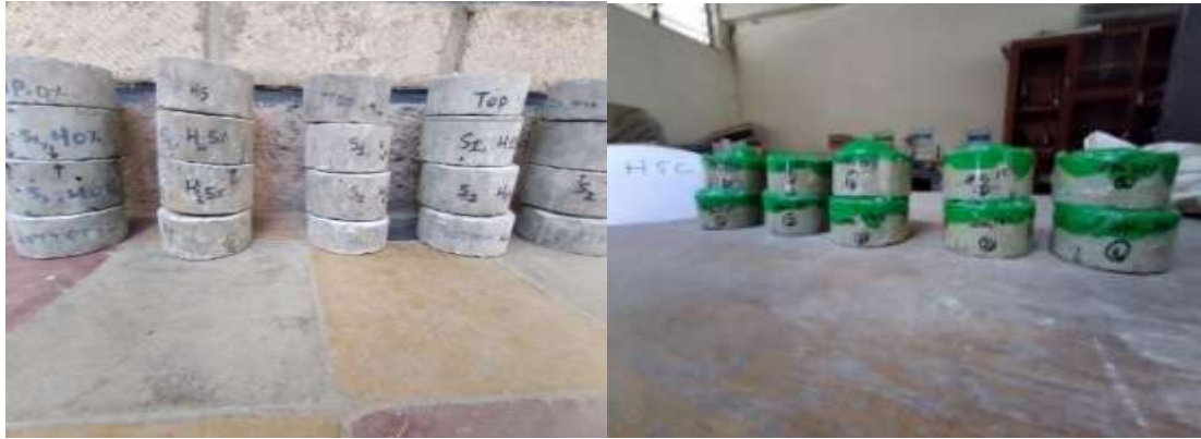
Figure 2. Sorptivity test specimens after cutting cylinder.
