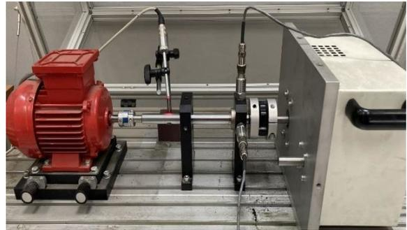
Figure 1 Experimental test-rig of PT 500.12
