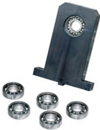
Figure 2 Six types of Bearings (SKF 6004) with different health status
